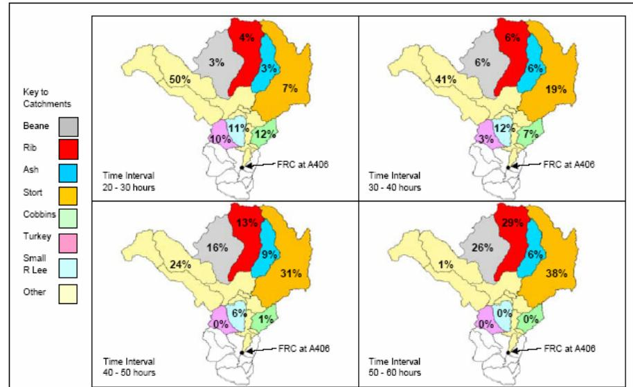
Figure 2.36 Breakdown by source of volume at the A406 (RLFRC) for a 1% AEP modelled event
